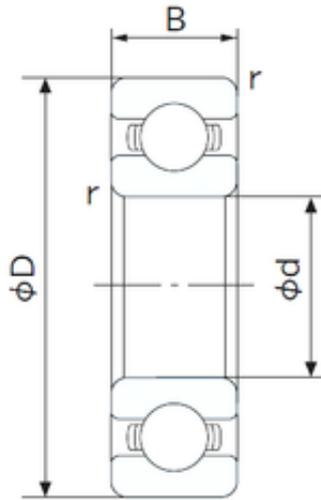
6000 Bearing 2D drawings and 3D CAD models
